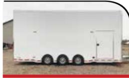
**2020 ATC Stacker Trailer** - Aluminum floor, removable fender, rear ramp door and a premium escape door!
